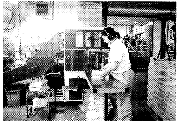
Stacking machine delivers bundles, ready to be put on pallet.
